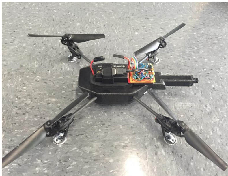
Fig. 9.2. Modified Parrot AR drone with Arduino micro
